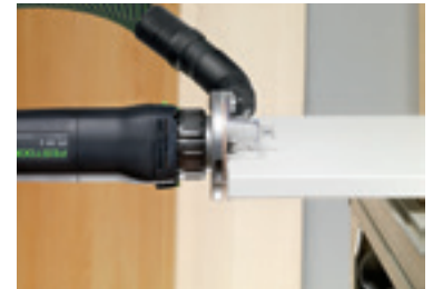
Rounding plastic or solid wood veneer.
