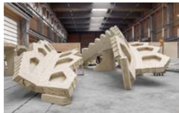
↑ Two industrial robots manufactured 376 different tile segments with 17,000 different finger joints.
