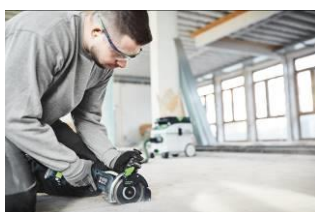
Image: Festool_DSC-AGC18FH_04.jpg The new Festool DSC-AGC 18 FH cordless freehand cutting system is being launched with an 18 V Bluetooth® battery pack and allows for dust-free cutting of mineral-based materials on the construction site.
