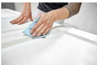
Image: Festool_Sanding_Know-How_19.jpg If necessary, hard-to-reach areas on profile grooves and transitions can be resanded using the extremely adaptable abrasive sponge
