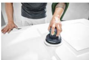
Image: Festool_Sanding_Know-How_18.jpg The ETS EC 150 eccentric sander and GRANAT abrasive with grit P240 to P500 is suitable for intermediate sanding
