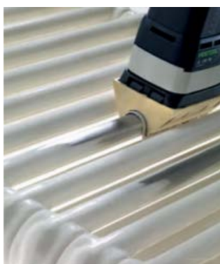
Image: Festool_Sanding_Know-How_23.jpg You can create an individual sanding pad using the DIY construction kit.
