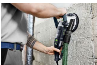
Image: Festool-RG130ECI-16.jpg Efficient dust extraction: Uneven substrates may cause leaks between the brush ring and the material. To prevent this from happening, the brush ring adapts to the surface being sanded and therefore ensures excellent extraction.
