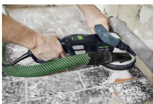
Image: Festool-RG130ECI-15.jpg Depending on the material and requirement, the speed of the RG 130 ECI can be individually adapted.
