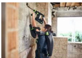
Image: Festool-ExoActive-A-05.jpg The ExoActive exoskeleton gives users an added boost before their arms get tired and at the same time takes the load off their neck.
