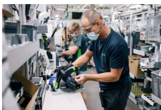
Image: Festool-new-building-Weilheim-06.jpg TS 55 plunge-cut saws are also manufactured on the new assembly islands in Weilheim an der Teck.
