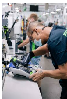
Image: Festool-new-building-Weilheim-08.jpg TS 55 plunge-cut saws are also manufactured on the new assembly islands in Weilheim an der Teck.
